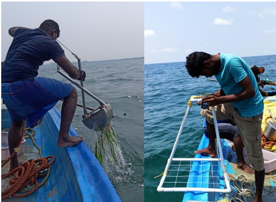
Figure 3.4a (left) Collection of sediment and seagrass sample using Van Veen Grab Figure 3.4b (right) Collection of quadrat data using a drop-down camera at Tamilnadu
