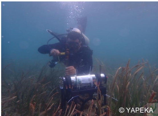
Installing BRUV cameras at a test site in Bahoi, North Minahasa
